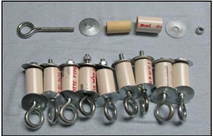
Ten alignment pins needed for the four home layout modules.
