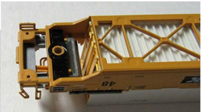
There is a very thin brace across the end of the well car that causes the interference with the Micro-Train truck. There is not much other support structure there, so cutting the brace out did not seem to be a good option. It would also take a lot of work to build the car up to take a body mount coupler.
