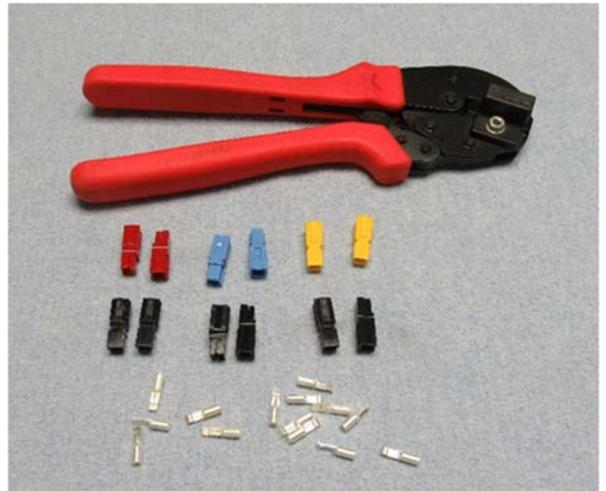
1. Strip the ends of the bus wire about 3/8 inch, just enough so that it fits all way into a power pole connector.
