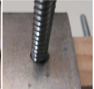
A number 10 sheet metal screw is the correct size.
