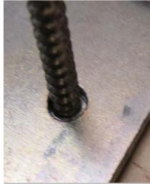
Dry wall screw does not fill the hole.
