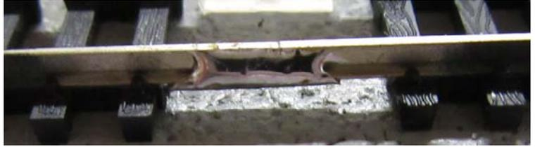
3. Inspect the joint and make sure it is soldered to both rails. Touch it up if necessary.
